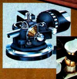
Unique Vario-pulley used in Dual's three belt-drive models is precision-machined for perfect concentricity and balance. Speeds are adjusted by expansion and contraction of pulley circumference; belt is never twisted or distorted.
